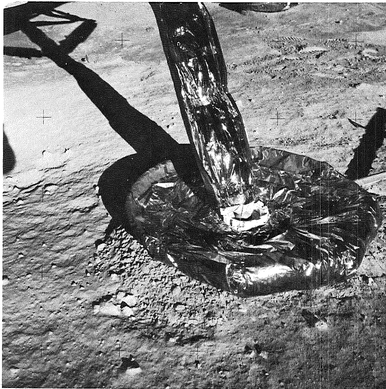
FIGURE 1-28. — The LM footpads were also photographed for later study of the surface mechanical properties. The foil wrapping provides thermal insulation. (NASA AS11-40-5926)
